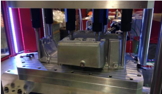
Pallet base with front O-ring to allow the pallet changeover without the need to unplug any pipes.
