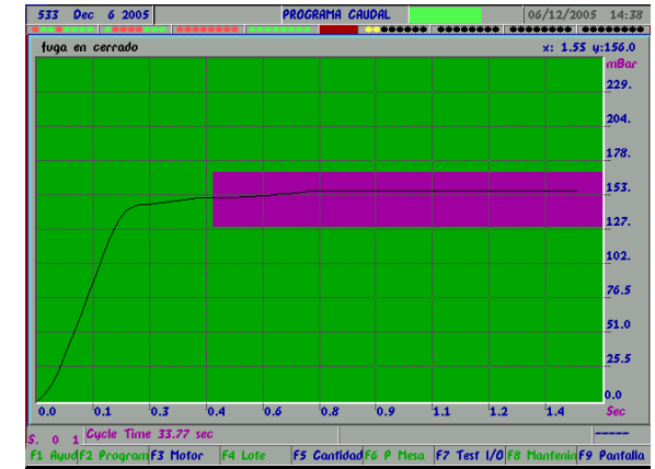
Leak test real time graphics.
