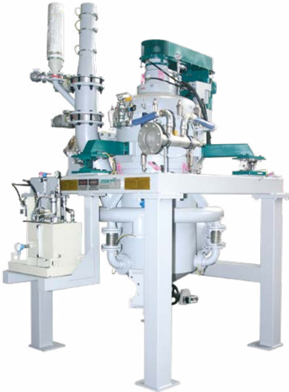
Fluidized Bed Jet Mill Type CGS 71 with oil circulating lubrication for hot gas operation
