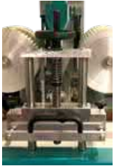
The feed system consists of gummied transport roller. The side fenders and top pressure systems are easy to adjust.
