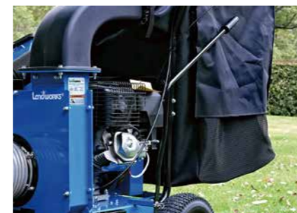
The control lever enables forward and reverse operation of the machine
