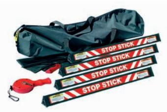
When driven over, the points of the STOP STICK® puncture the tyres and the Teflon® coated metal tubes penetrate the tread. The air is released unhindered Deflation takes an average of twenty to thirty seconds. The vehicle retains directional stability and can be safely brought to a stop
