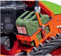
Removable-fuel-tank-system by Agria, fuel level display on remote control
