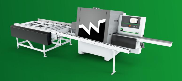
From small strips to large beams: with the Cube 3 you can plane a vast range of dimensions – without any prior technical knowledge, and all in efficient one-man operation. This is made possible by the high level of automation present in the automatic planer, which is reflected in optional features such as the WEINIG automated stacker or the RFC 15 return conveyor.
