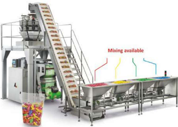
RM-25ACC With a product mixing system
