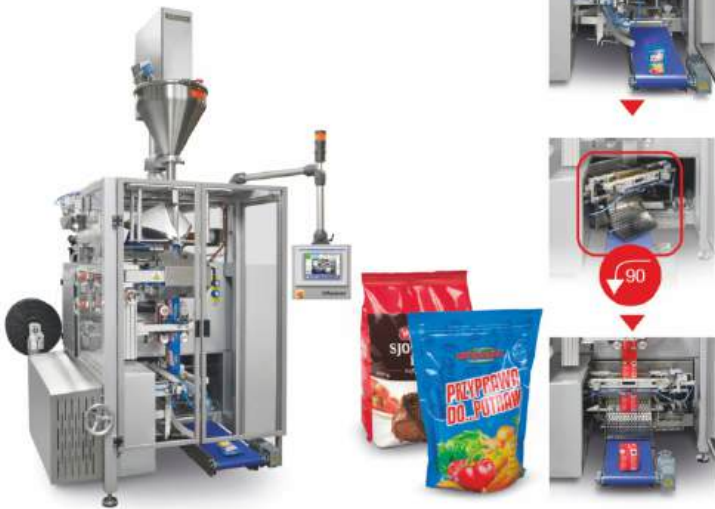
RM-32ACD Doypack bagger with rotatable horizontal jaws and zipper applicator
