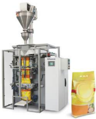
RM-45AC With servo auger doser
