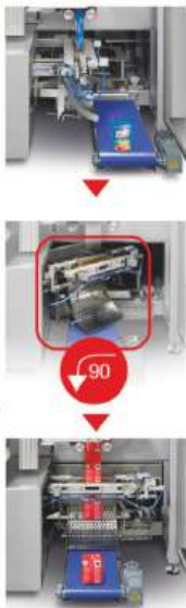
RM-32ACD Doypack bagger with rotatable horizontal jaws and zipper applicator
