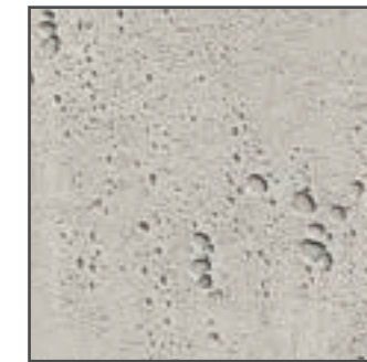
120 Beton Glatt. grau | concrete smooth form.
