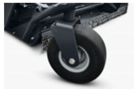
The run-flat tyres provide extended reliability when working 2+3
