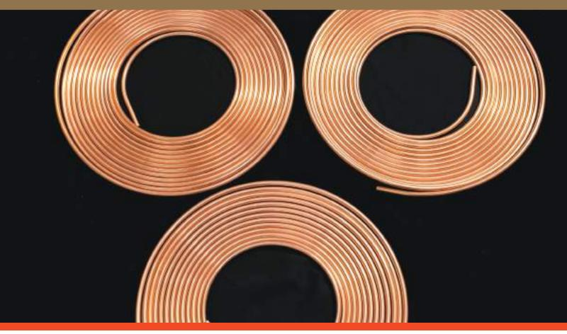
UCI manufactures pancake coils with diameters ranging from 4.76 to 22.22 mm and thicknesses between 0.30 to 1.20 mm.
