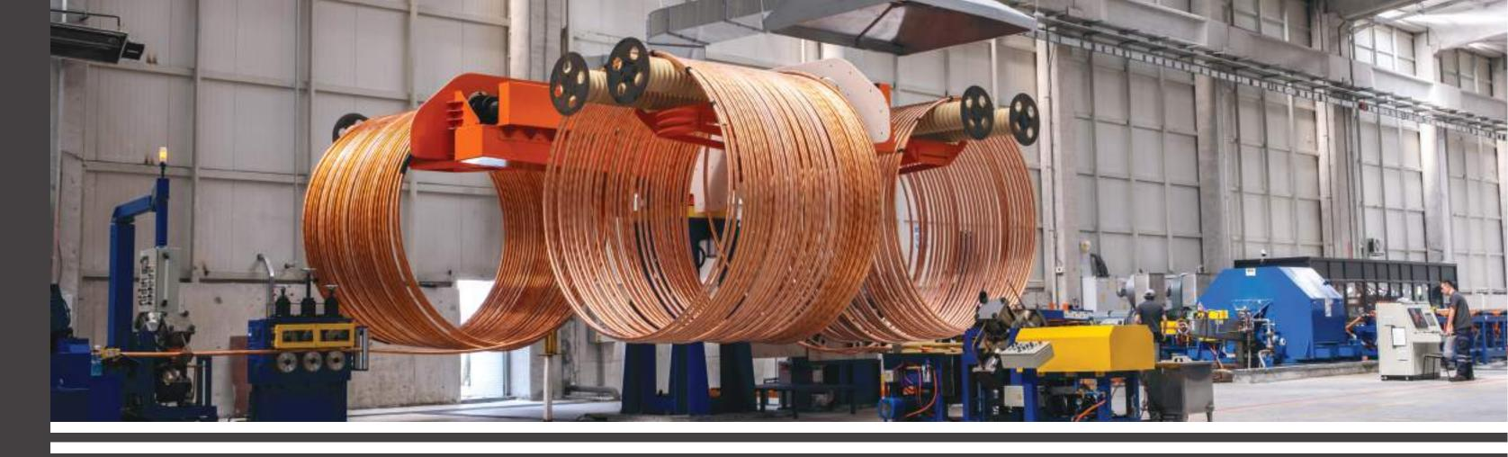
At UCI facilities, production is carried out using the Cast & Roll continuous casting technique, utilizing high-quality copper cathodes sourced from leading copper cathode manufacturers worldwide, without incorporating scrap copper usage. A wide range of copper tubes with superior properties, produced to meet the needs of different industries, is offered in product types such as LWC, straight-length, pancake coil, and grooved tube, tailored to their respective purposes.
