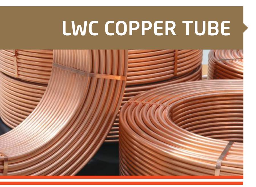
UCI copper tube production is carried out with diameters ranging from 4.76 to 22.70 mm and wall thicknesses between 0.30 to 1.20 mm, in annealed and hard tempers.
