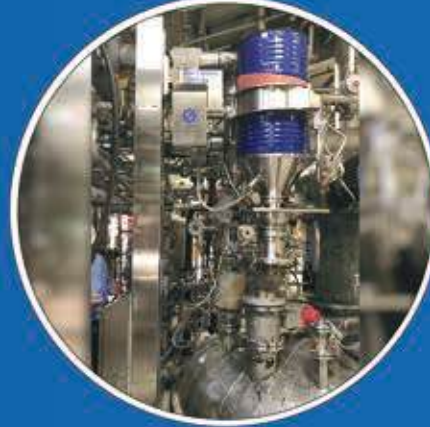
Fixed Automatic Drum Lifter for Reactor Loading
