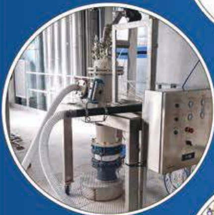
Coated VTS model AGR250KK for reactor loading with solvents and acids.
