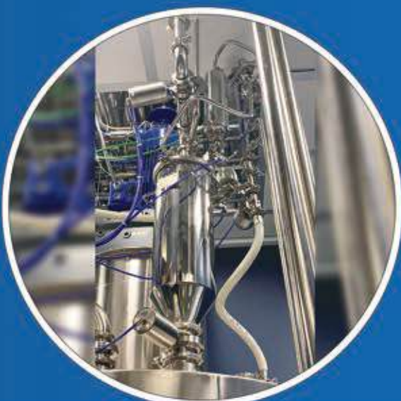
Filtervac FT200 for reactor charging
