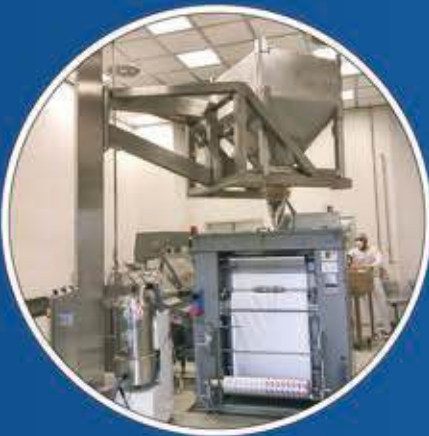
Bin Lifting Column connected to the sachet packaging machine
