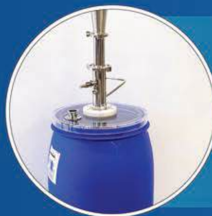
Suction Lance connected to a drum with a cap, thus creating a closed system preventing the product from escaping into the working area
