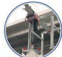
Used to lift and position Big Bags without using the forklift
