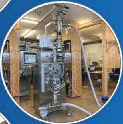
Vacuum Conveyor to load a Roller Compactor
