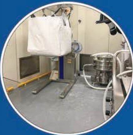
Mobile Lifting Column for Big Bag Unloading
