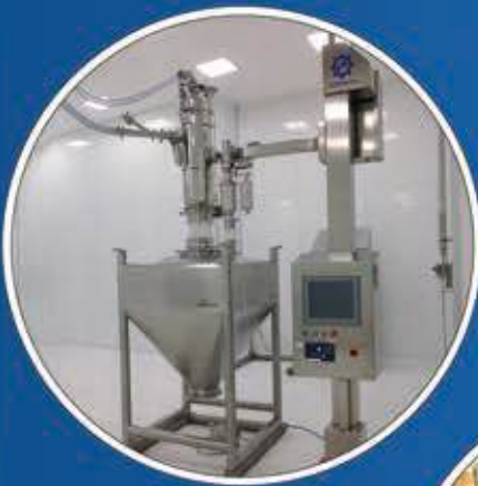
Vacuum Conveyor to load a Roller Compactor
