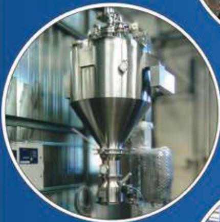
VTS Hoppervac with integrated washing system for chemical application
