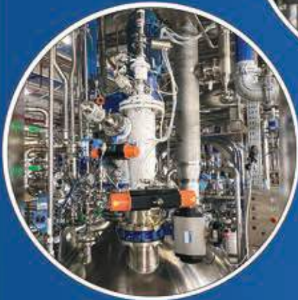
VTS model AGR250KK PN6 for reactor loading from Glove Box OEB4 for API
