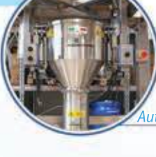
Suction hopper It is installed on the Big Bag Discharge Station outlet point and creates a closed system, allowing direct powder transfer by vacuum from the Big Bag into the other machinery
