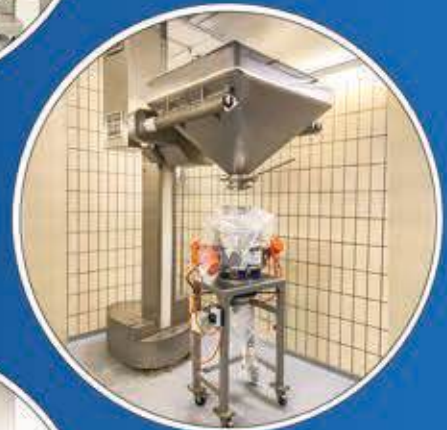
Bin Blending Column for Mill loading
