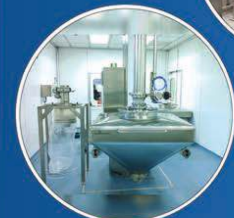
Bin Blending Column for Mill loading
