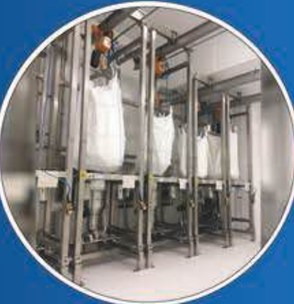
Integrated Big Bag Unloading System with Vacuum Conveyor for Bin
