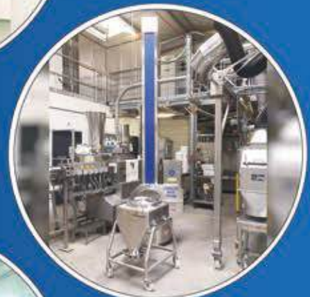
Blender Column with Clamp Connection for Bins with removable trolley
