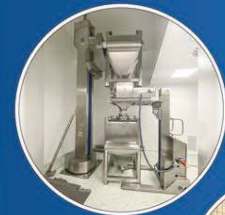
Blending and discharging System from Bin-to-Bin by Mill
