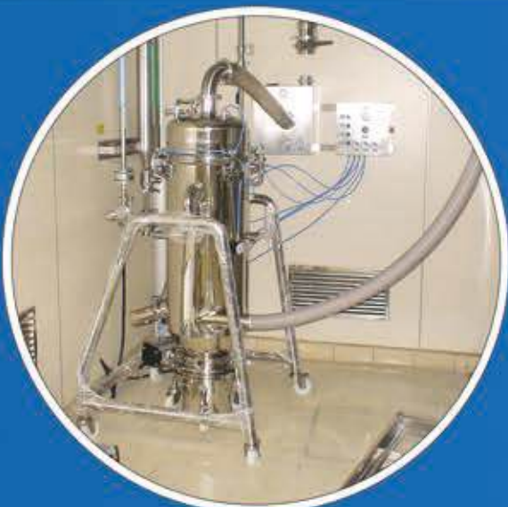
Filtervac FT400 for Bicone loading
