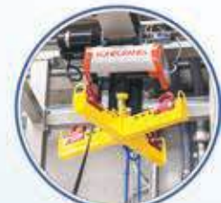
Used to attach and support the Big Bag
