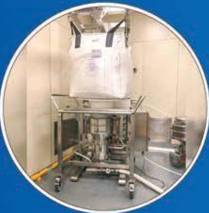
Mobile Closing System integrated with CIP
