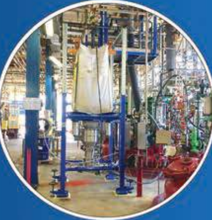
Big Bag Discharge Station for feeding reactor using Vacuum Conveyors
