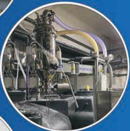
Vacuum Conveyor on a arm for charging a silo
