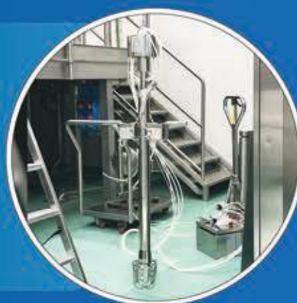
Lump Breaker Lance with spring balancer
