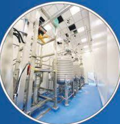
Big Bag Discharge Station for feeding dissolvers using Vacuum Conveyors
