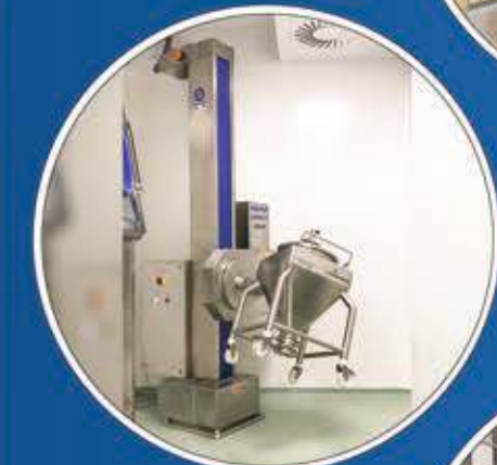
Fixed Bin Blender Column with Clamp Connection for Bin connection
