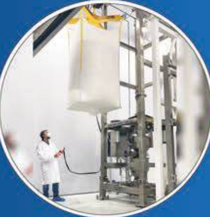
Big Bag Discharge Station installed on load cells
