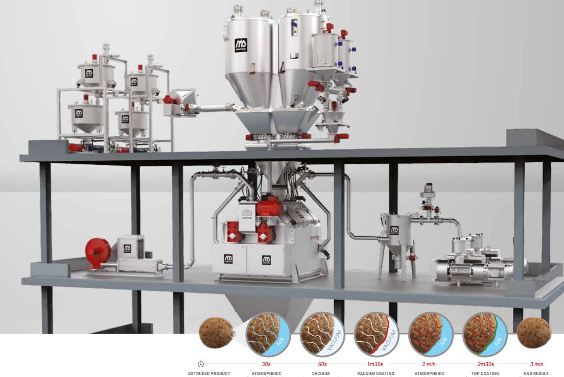
Product is fed into the Pegasus Vacuum Coater in atmospheric conditions A vacuum is created inside the Pegasus
