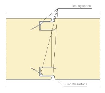
Intelligent panel joint construction makes assembly and operation more efficient.
