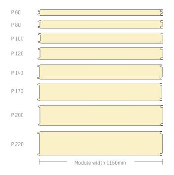
Available in eight economical insulation thicknesses, depending on the desired operating temperature.
