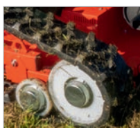
Crawler tracks with non-slip cleat-profile
