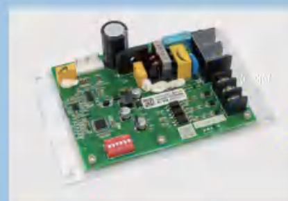
外置三速风机驱动器 - 200W External Three-Speed Fan Motor Driver - 200W
