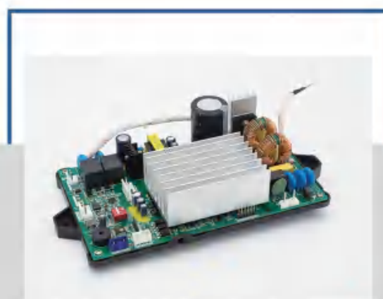
变频油烟机驱动 - 500W Inverter Range Hood Driver-500W
