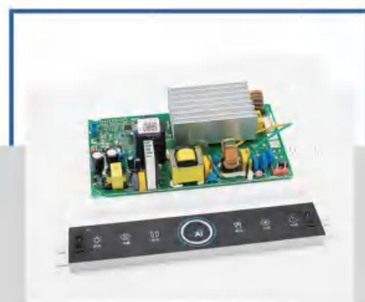
变频油烟机控制&驱动 - 300W Inverter Range Hood Control & Driver-300W
