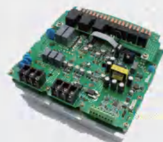
三相变频水泵驱动器 - 22kW 3-Phase Inverter Water Pump Driver-22KW
