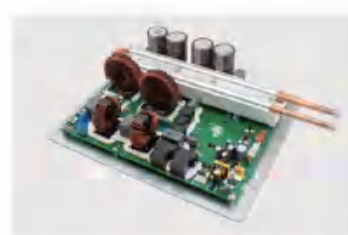
SPB1-D26080BA1-单相冷媒驱动器 - 8KW 1-Phase Refrigerant Cooled Driver - 8KW
