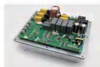
SPB1-D38120AA1-三相无电解驱动器 - 12KW 3-Phase No Electrolytic Driver - 12KW
