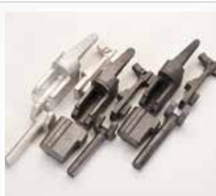
Bascule, sottoguardie, croci e monoblocchi ricavati da masselli forgiati Action bodies, trigger plates, iron fore-ends and barrel extractors pieces are milled from forged steel ingots. Bascules, sous-gardes, monoblocs et longuesses usinés à partir de blocs forgés
