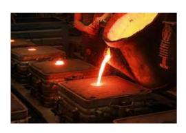
This type of casting method creates a sand mould, into which the molten metal is then poured. When the metal finishes the cooling process, the outer mould will break. The sand can be reused to create another mould, whereas a mould can only be used once. Sand casting is widely used to cast large metal parts, and the lower cost is the advantage of mass casting.
