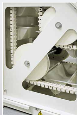
Transition from horizontal to vertical conveying
