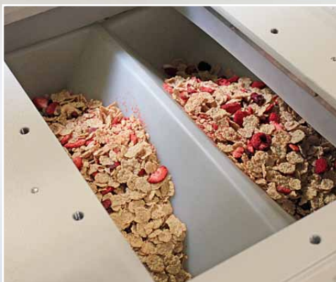
Feed point with silicon seal
