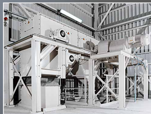
Discharge section of a WB 640 with 30 kW drive
