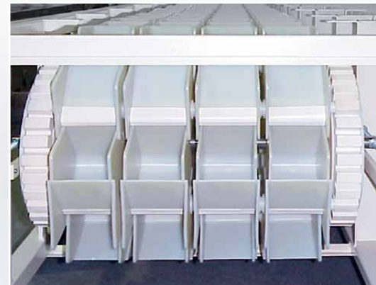
Multiple bucket belt at the tensioning unit
