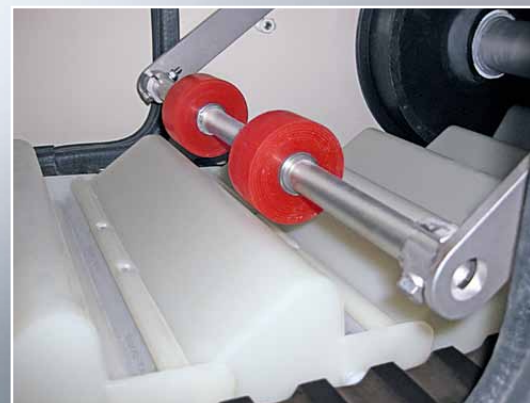
Pendulum bucket knocker to assist product discharge
