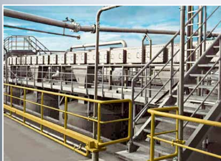
Gas-tight horizontal pendulum bucket conveyor
