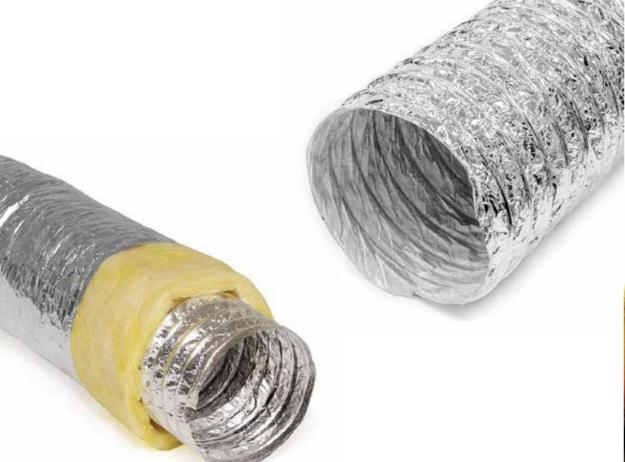
Highest quality flexible ducts can be produced by permanently bonding laminates of Aluminium Foil/Polyester Film to a spring steel wire helix.
