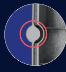
► 02 Occlusions= Checking the opening of holes and interception of occlusions (even partial) due to the presence of burrs or broken plugs
