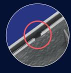
► 04 Lack or = abundance of material Identification of material excesses or lacks due to molding or shearing problems
