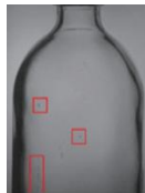
Surface Defect Detection of Transparent Bottle
