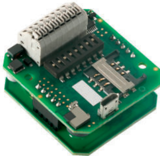
TWN4 Palon Compact M* Full version: 125 kHz, 13.56 MHz, NFC, BLE
