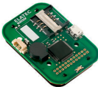
TWN4 MultiTech 3 M* Full version: 125 kHz, 13.56 MHz, NFC, BLE Available in different combinations
