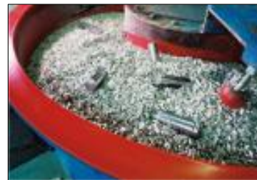
Deburring processes and part cleaning
