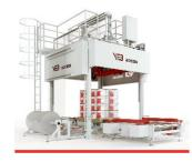
FB 1000 AVAILABLE IN 4 VERSIONS: SMALL-STND-XL-XXL MAX PALLET SIZE 2600x1400mm CAPACITY: 70 PALLETS/hr PATENTED SYSTEM
