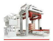
STARSTRETCH FB4.0 AVAILABLE IN 6 VERSIONS: SMALL-STND-L-XL-XXL-XXL+ MAX PALLET SIZE 3600x1700mm CAPACITY: 280+ PALLETS/hr ALL OPERATIONS AT FLOOR LEVEL PATENTED SYSTEM
