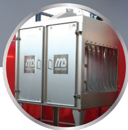
This Bag Cleaning Cabinet disinfects bags using ozone
