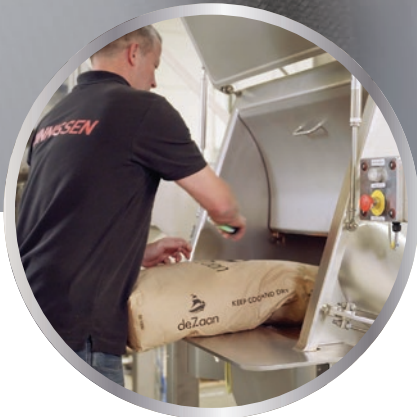
Operator opens a bag in a Dima® MAN
