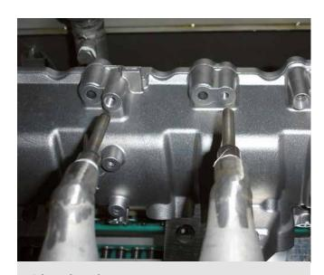
**Adapted nozzles** for targeted air blast cleaning of holes
