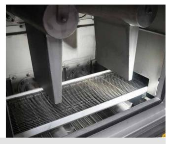
for flat components with air blast nozzles only from top and bottom
