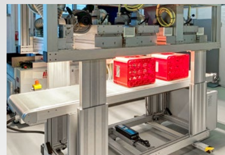
Drying with a "Multiple-IR-Curing" NIR module.
