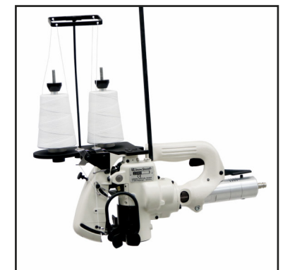
2200L,LA Air-motor driven single or two thread portable sewing machine with special top and bottom feed for closing bags in hazardous locations (dust explosion).
