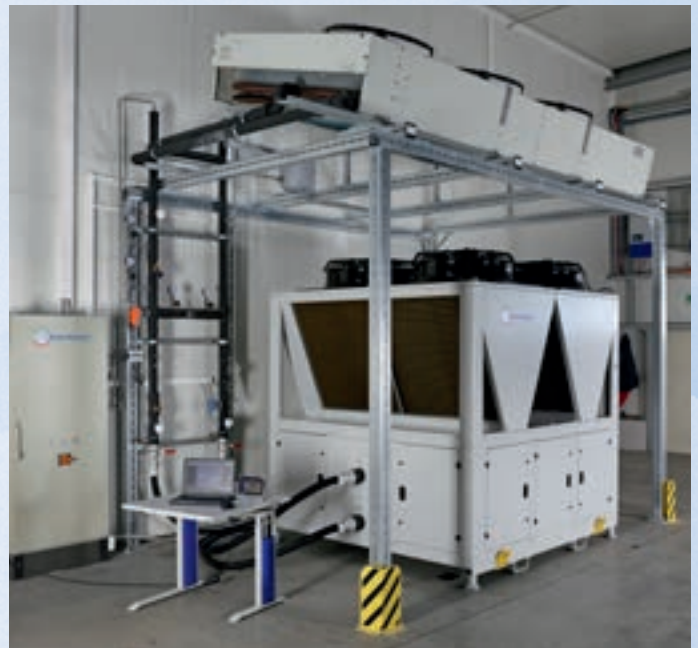
In-house machine test bench for testing and continuous development of the machines. Newly developed control concepts can be tested comprehensively by us.
