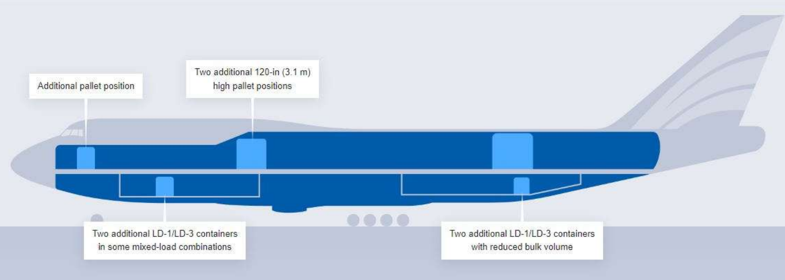
Cross Section Showing Main Deck and Lower Compartment
