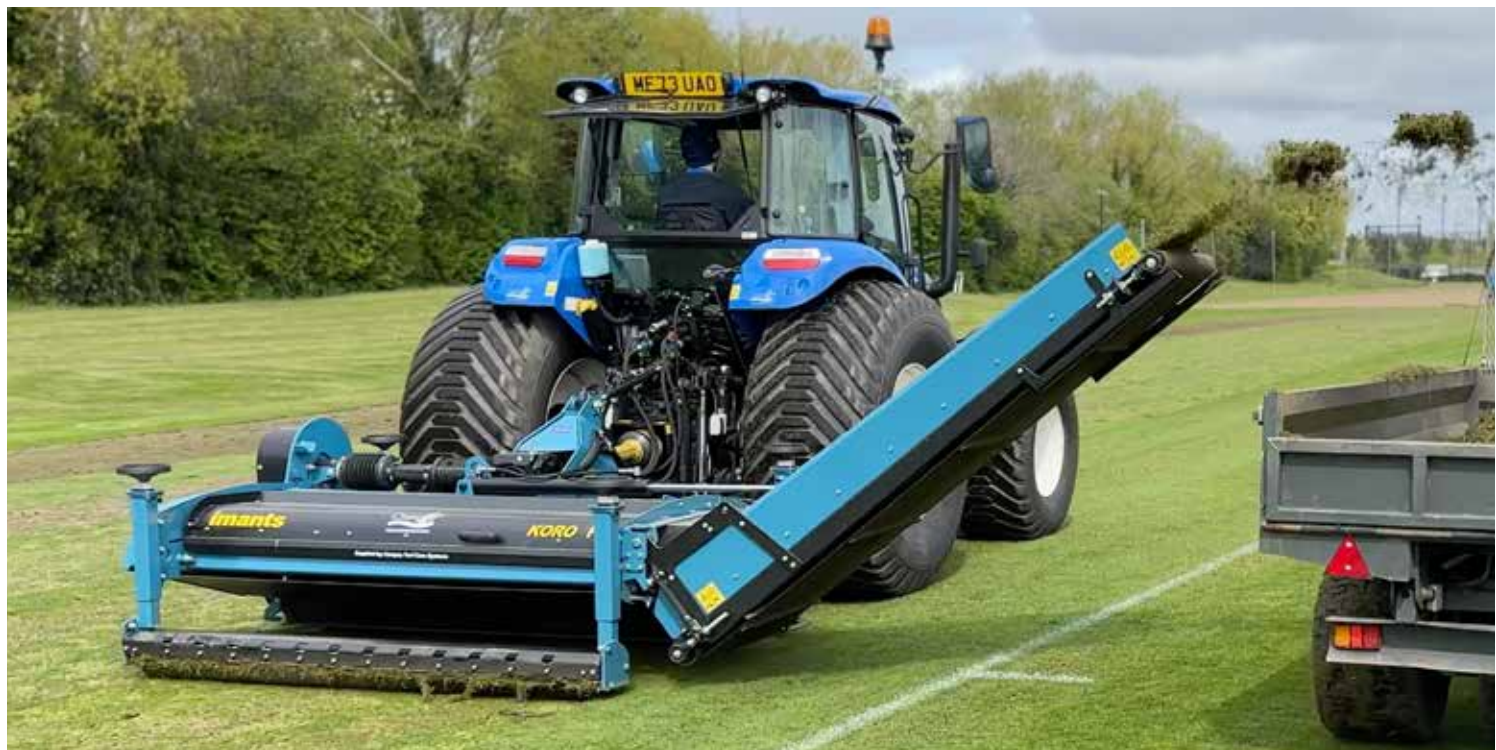
The UNIVERSE® rotor was initially developed for the removal of organic build up from the surface of semi-synthetic natural turf pitches that are now common in professional stadiums around the world.
