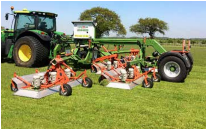
Fleischmann electric 5 Deck Rotary Mower with 2.20m cutting decks.
