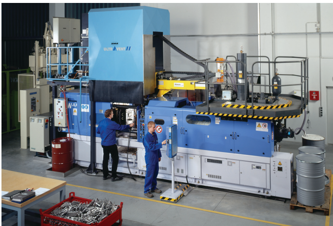
Figure 4: 220 t-Thixomolding-Maschine (JLM220MG, Japan Steel Works Ltd.) at NMF.
