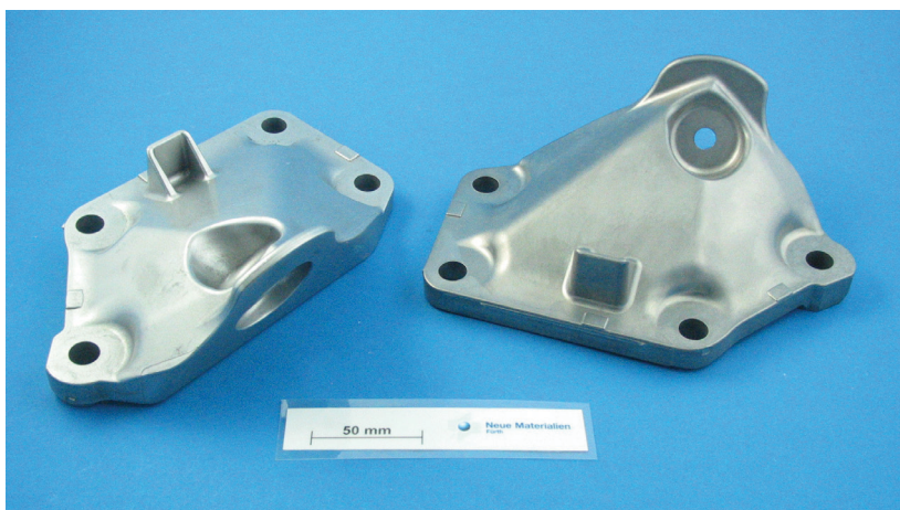
Figure 2: The porosity of thick walled parts like an engine bracket can be reduced significantly by using magnesium injection molding in comparison to die casting.
