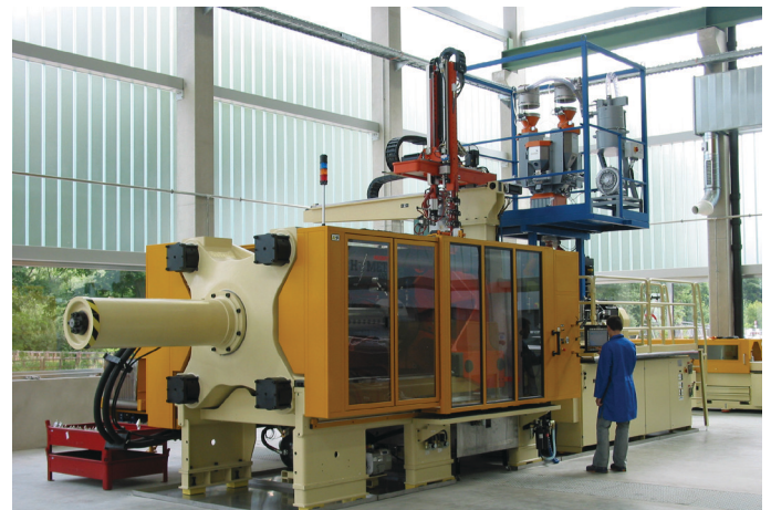
Figure 5: 650 t-Thixomolding-Maschine (HyMet650, Husky Injection Molding Systems Ltd.) at NMF.
