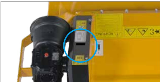
V-belt tension is always visible: V-belt protection with inspection opening.
