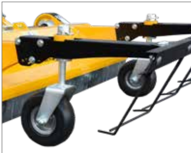
Vertically adjustable support wheels, 360-degree swivelling
