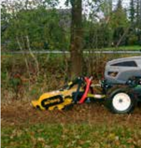
The MU-C for front mounting: Low coupling points and a low-mounted gear box (input speed of 1000 or 2000 rpm).
