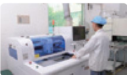
AUTOCK AT-320 Automatic Optical Depaneling Machine
