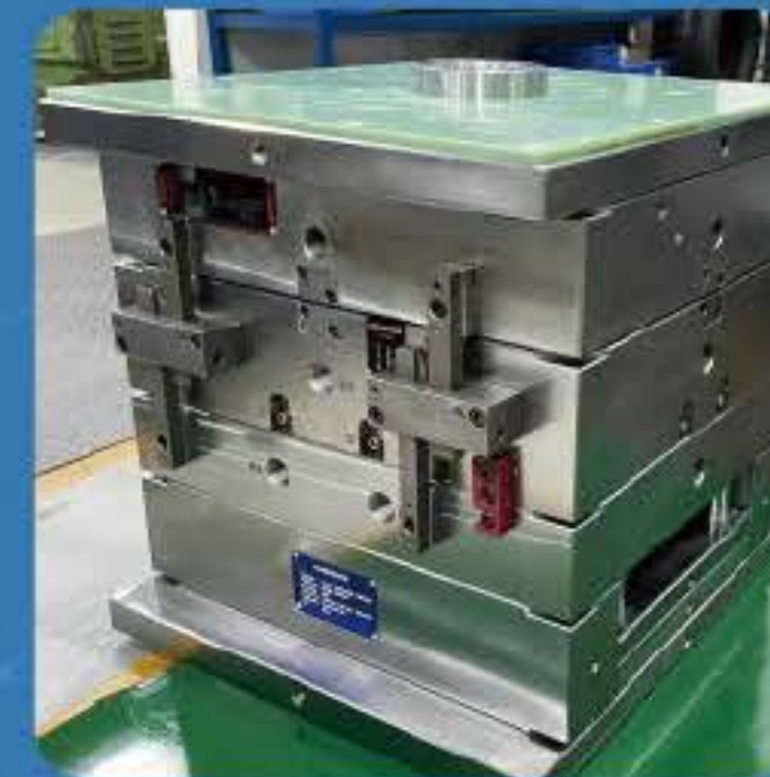
HASCO standard single nozzle hot runner mold
