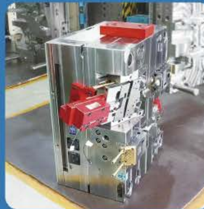
Precision tube mold with core pulling structure
