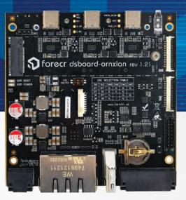
DSBOARD-ORNX-LAN is an industrial carrier board designed for harsh environments and applications that demand high processing power and reliability. It is based on the NVIDIA Orin NX system-on-module (SOM), which features multiple NVIDIA Ampere GPU cores and Arm64 CPU cores. The compact design of the carrier board makes it a versatile and flexible solution for a wide range of industrial applications such as autonomous systems, robotics, and intelligent video analytics.
