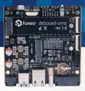
DSBOARD-ORNX is an industrial carrier board designed for harsh environments and applications that demand high processing power and reliability. It is based on the NVIDIA Orin NX system-on-module (SOM), which features multiple NVIDIA Ampere GPU cores and ARM64 CPU cores. The compact design of the carrier board makes it a versatile and flexible solution for a wide range of industrial applications such as autonomous systems, robotics, and intelligent video analytics.
