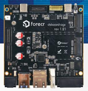
DSBOARD-AGX is a powerful and reliable edge computing device designed for industrial applications that require high processing power and ruggedness. It is based on the NVIDIA Jetson AGX Orin systemon-module (SOM), which features an NVIDIA Ampere GPU with 1024 CUDA cores and up to 275 TOPS (trillion operations per second) of AI performance. The AGX Orin SOM also includes a 12-core ARMv8.2 CPU and a dedicated deep learning accelerator for efficient inferencing.
