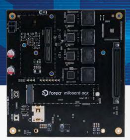
MILBOARD-AGX is a carrier board designed for harsh military and aerospace environments. It is powered by the NVIDIA Jetson AGX Xavier module, which has an NVIDIA Volta GPU and an eight-core ARM64 CPU, providing high processing power for complex applications. The carrier board features a rugged design that ensures reliable performance even in the most extreme conditions. It has a wide operating temperature range and a robust power management system that can handle input voltages from 18V to 32V.
