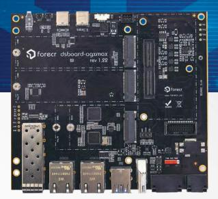
Introducing the DSBOARD-AGXMAX, the industrial carrier board that is built to maximize your productivity and connectivity. Powered by the high-performance AGX Orin SoM, which can deliver up to 275 TOPS of AI performance, this board offers top-of-the-line 10G connectivity, as well as Dual Gigabit Ethernet, USB 3.2, HDMI, CAN, Serial Ports, and MIPI CSI-2 Camera support.
