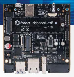
The DSBOARD-NX2 is a carrier board designed to support the NVIDIA Xavier NX, Jetson Nano, and TX2 NX System on Modules (SoMs) for advanced edge computing applications.
