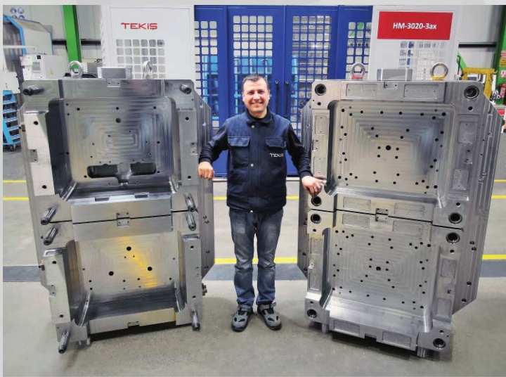
2200 x 3200 mm - 30 tons part machining
