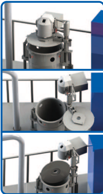
Melting chamber and nozzle plate can be raised and turned to the side independently. Rotatable nozzle plate.
