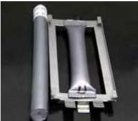
Zero hour sample (prior to exposure) and a sample subjected to an accelerated ageing test after 4.000 hours of exposure.
