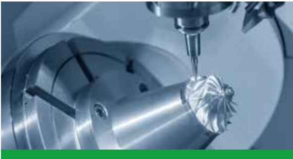
CNC Machining Milling (3-, 4- & full 5-axis), turning & post processing
