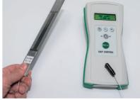
The Gap Gauge GAP CONTROL is a technical innovation which makes everyday tasks during machine assembly easier. The GAP CONTROL has been developed in order to precisely determine typical gaps starting at 1.8 mm between hard pairs of rollers or cylinders. At the same time, the device is able to determine the width between slots or slits in mechanical components.
