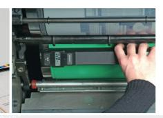
The LUCHS Register Measuring System is today used worldwide for the quality control, adjustment and error analysis of printing presses. It is able to measure the transfer, front-to-back and feed register of multicolour printing presses. Optionally, the device can be used to measure the varnish, the folding and cutting register. The measurement is carried out by recording and analysing special measuring elements located at different positions on the printed sheet.
