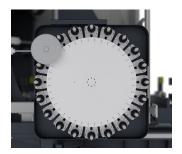
High speed rates on axes and internal automatic tool replacement magazine which moves with gantry for 20+1 tools allow for time savings when running different processes which require tool replacement.
