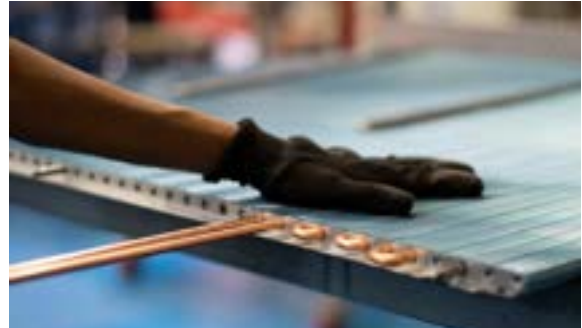
Hairpin tubes fitted in fins
