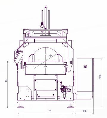
\* adjustable between 45 mm and 115 mm the drawing shows optional equipment Dimensions in mm Technical changes reserved
