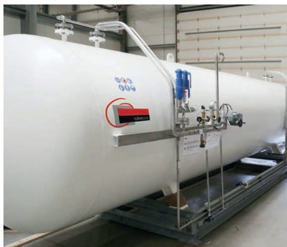
Figure 2. CO 2 high-pressure tank.
