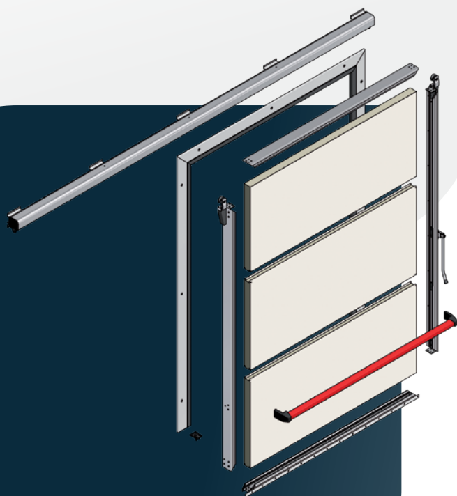
Standard 100 mm (KH-1010/PKD-100s)/140 mm (VH-1414) sandwich panel applicable
