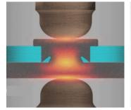
The light-weight component is welded to steel component in the body shop using standard welding equipment
