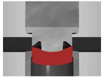
The light-weight component is pre-equiped with ERWin® via post operation crimping without prehole (above) or in-die/in-mould
