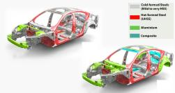
The ERWin® multi-material welding insert is compatible with existing body-shop welding equipment AND with all multi-material combinations, so enabling all levels of light-weight material use in body-in-white designs to co-exist on the same assembly line, without additional investment, from all-steel to advanced multi-material bodies.
