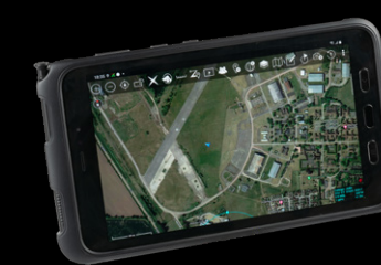
ATAK on Android End User Device (EUD) with Thermoteknix ARTIM plug-in
