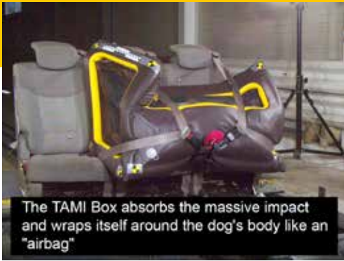
Then the TAMI Box springs back into its original position. The test was performed several times!
