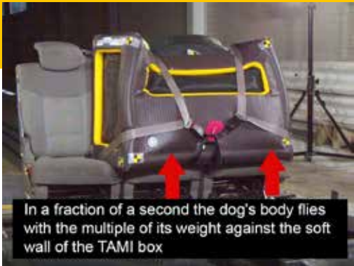
The TAMI Box absorbs the massive impact and wraps itself around the dog's body like an "airbag"
